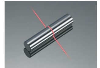
Profile measurement of a metal pin-gage
