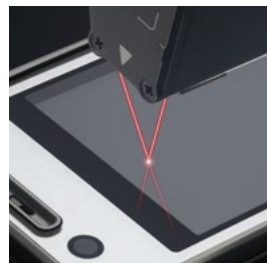
Measurement of the touch panel surface height and air gap.
