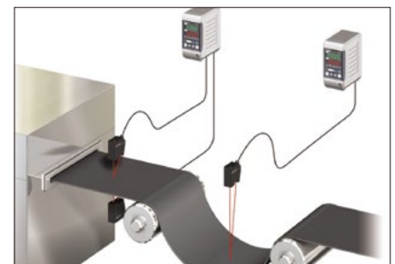
Thickness measurement/loop control of a rubber sheet
